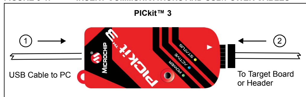
FIGURE 3-1: INSERT COMMUNICATIONS AND USB/POWER CABLES
