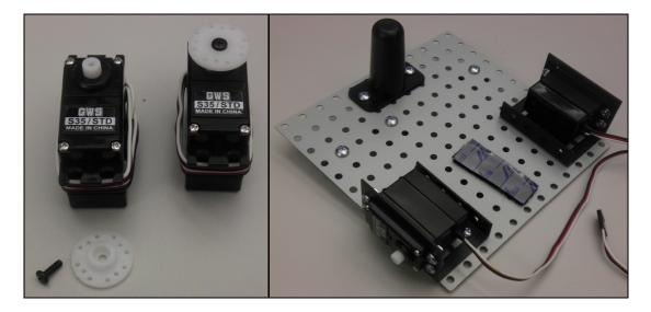
7. Take out the two wheels and the rubber traction bands. Stretch the rubber band around the outside of the wheel. Then, attach the wheels to the servos, and secure them using the small black screws that were removed in the previous step.
