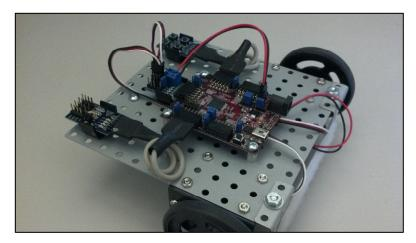
17. Attach the four IROS to the bent bracket from left to right using the attached Velcro, and connect the sensors in the same order to each of the headers (S1-S4) on the PmodLS1. In other words, if the robot is facing forward, and you are looking down on it from above, the sensor on your far left should be connected to S4, the sensor at mid left should be connected to S3, the sensor at mid right should be connected to S2, and the sensor at the far right should be connected to S1.
