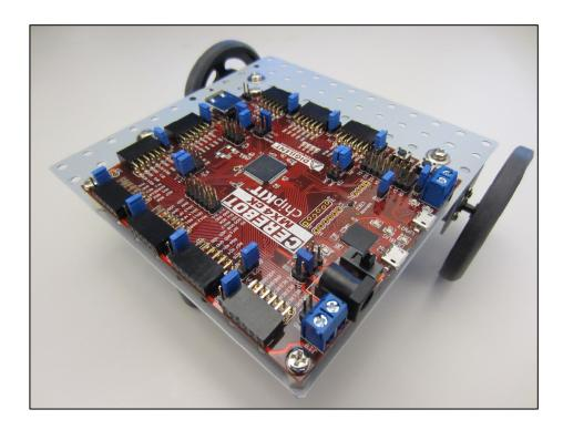
9. Connect the two PmodHB5 modules to port JD on the Cerebot MX4cK board using the two 6-pin cables. Using the PmodHB5s, connect the left motor to the bottom row of JD, and the right motor to the top row of JD. Use the marker on the cable connector to ensure that pin placements are in alignment when connecting the boards. See the pictures below.
