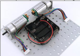
4. Attach the Pmod clips to the metal platform on both sides of the battery holder.
