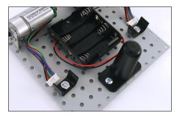
6. Attach the two PmodHB5 modules to the Pmod clips and connect them to the motors.
