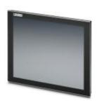
19-inch/48 cm flat panel LCD monitor with resistive touch screen. Includes two rear USB ports
