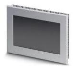
Touch panel with 17.8 cm/7" TFT-Display (Resistive industrial touch screen), 800 x 480 Pixel (WVGA), 262144 colors, ARM® Cortex®-A8, 800 MHz, 2x USB Host 2.0, 1 x Ethernet (10/100 Mbps), RJ45, Debian GNU/Linux and User software: Midori Browser. (Bus system: without)
