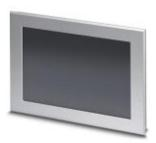
Touch panel with 30.7 cm/12.1" TFT-Display (Resistive industrial touch screen), 1280 x 800 Pixel (WXGA), 16.7 million colors, ARM<sup>®</sup> Cortex<sup>®</sup>-A8, 800 MHz, 2x USB Host 2.0, 1 x Ethernet (10/100 Mbps), RJ45, Debian GNU/ Linux and User software: Midori Browser. (Bus system: without)
