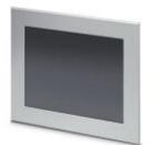
Touch panel with 26.4 cm/10.4" TFT-Display (Analog resistive (polyester)), 800 x 600 Pixel (SVGA), 262144 colors, ARM<sup>®</sup> Cortex<sup>®</sup>-A8, 800 MHz, 2x USB Host 2.0, 1 x Ethernet (10/100 Mbps), RJ45, Windows<sup>®</sup> Embedded Compact 7 and User software: Visu+ / AX OPC Server. (Bus system: without)
