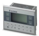
Key panel with 7.6 cm/3" FSTN-Display (without), 160 x 80 Pixel, 5 grayscales, ARM9<sup>™</sup>, 200 MHz, 2x USB host 2.0, 1 x Ethernet (10/100 Mbps), RJ45, Windows CE 5.0 and User software: TSvisRT. (Bus system: PROFIBUS DP)
