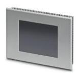
Touch panel with 14.5 cm/5.7" TFT active-display (analog resistive (polyester)), 320 x 240 Pixel(s) (QVGA), 65536 colors, ARM9<sup>™</sup>, 200 MHz, 2x USB host 2.0, 1 x Ethernet (10/100 Mbps), RJ45, Windows CE 5.0 and user software: TSvisRT. (bus system: MPI)
