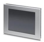
Touch panel with 26.4 cm/10.4" TFT-Display (Analog resistive (polyester)), 800 x 600 Pixel (SVGA), 262144 colors, ARM® Cortex®-A8, 800 MHz, 2x USB host 2.0, 1 x Ethernet (10/100 Mbps), RJ45, Windows® Embedded Compact 7 and User software: IniNet Browser. (Bus system: without)
