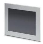
Touch panel with 38.1 cm/15" TFT-Display (Analog resistive (polyester)), 1024 x 768 Pixel (XGA), 262144 colors, ARM® Cortex®-A8, 800 MHz, 2x USB host 2.0, 1 x Ethernet (10/100 Mbps), RJ45, Windows® Embedded Compact 7 and User software: IniNet Browser. (Bus system: without)
