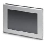
Touch panel with 22.9 cm/9" TFT-Display (Resistive industrial touch screen), 800 x 480 Pixel (WVGA), 262144 colors, ARM® Cortex®-A8, 800 MHz, 2x USB Host 2.0, 1 x Ethernet (10/100 Mbps), RJ45, Debian GNU/Linux and User software: Midori Browser. (Bus system: without)
