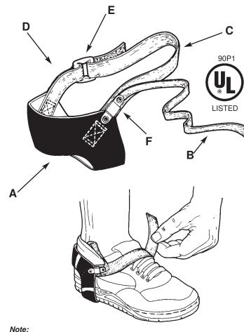
Two heel straps are recommended for reliable grounding and ESD protection, providing ground when one foot is off the floor.
