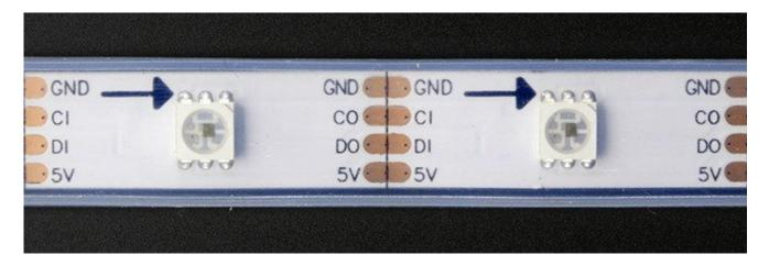
First, look for arrows printed along the strip next to each LED. These show the direction of data moving down the strip...your microcontroller connects at the originating ("in") end, the arrows point toward the "out" end. (In the photo above, our microcontroller would be located off the left side.)
