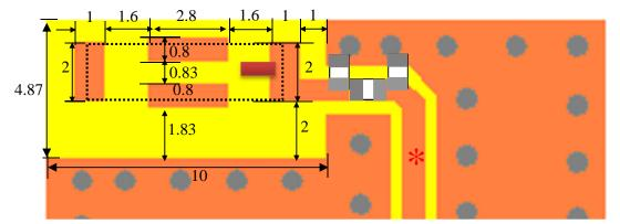
IMPORTANT! Matching circuit and component values will be different on your PCB, this will depend on PCB layout and shape, encasment, etc
