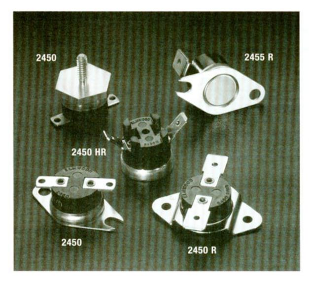
A temperature-sensitive bimetal disc, electrically and thermally isolated from the switch, is used to actuate the normally-closed contacts. Contacts are opened when surface or ambient temperatures increase to the operating snap point of the calibrated bimetal disc. The entire switch is enclosed in a phenolic dust-free housing; the bimetal disc is retained by a metal heat-conducting end cap.
