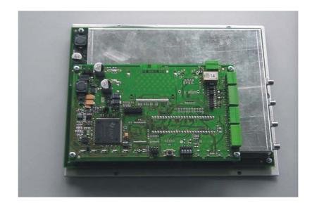
Multi-protocol Long Range Reader Module for identification of UHF transponders (865-928 MHz) in the fields of retail, industry, logistics etc.
