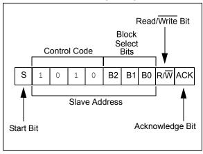
FIGURE 5-2: ADDRESS SEQUENCE BIT ASSIGNMENTS
