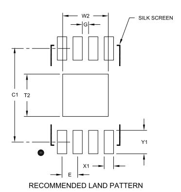
Units MILLIMETERS Dimension Limits MIN MAX NOM 0.50 BSC Contact Pitch Е Optional Center Pad Width W2 1.46 Optional Center Pad Length T2 1.36 Contact Pad Spacing C1 3.00 Contact Pad Width (X8) X1 0.30 Contact Pad Length (X8) <u>Y1</u> 0.75 Distance Between Pads G 0.20
