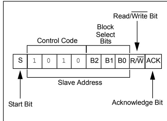
**FIGURE 5-2: ADDRESS SEQUENCE BIT ASSIGNMENTS**
