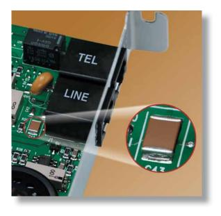
The Tip & Ring MLCC series are designed specifically for telecom ringer circuit applications where it is necessary to provide a block of the line voltage (typically -48 VDC) while passing the AC ringing voltage. These compact ceramic SMD chips replace bulky leaded film caps saving board space and stream-lining the assembly process.
