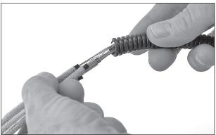
7.2 Route output tube(s) into desired splice tray(s).
