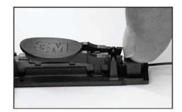
7.8 Grasp the left fiber about 2 inches from the holder and push the fiber in until it bows about 1/8 to 1/4 inch (3mm to 6mm). Push down on the actuation lever until the Fibrlok II Splice is actuated. An audible click can be heard and you should feel the splice cap snap down into place when completely closed. The cap should be level with the Fibrlok splice top surface.
