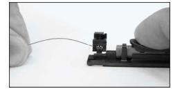
7.9 Release the bow in the fiber and fully close the left buffer clamp. Again, you will hear an audible snap.
