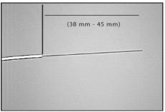
Note: Cleavers must be in good operating condition and used per the manufacturer's instructions. They should provide consistent cleave-to-coating lengths within +/-0.5mm. Acceptable cleavers will produce cleaved ends within  $0.5^{\circ}$  of perpendicular (typical always  $<1^{\circ}$ ), free from major defects.
