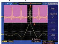
Use the oscilloscope's delayed sweep feature to zoom in on a particular area of a signal in real time while viewing the entire captured waveform simultaneously.
