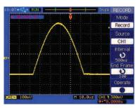
Monitor and analyze long term signal behavior by recording data continuously over an extensive period of time and playing it back for post acquisition analysis. Data is recorded in a sequence of up to 1000 frames of 4 k data points each and the time interval between each frame is adjustable from 1 ms  $-100\,\text{s}$ . The data can be saved in a single file to internal memory or USB flash drive.
