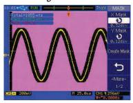
Create a user defined mask (pass/fail limits) and automatically compare it against the input signal from CH1 or CH2. This feature is ideal for manufacturing test applications that require instant go/no go test results.
