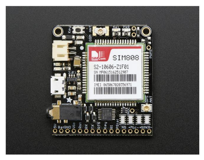
On its own, this module can't do anything. It requires a microcontroller to drive it! We suggest and use an Arduino but any 3-5V microcontroller with a UART can send and
