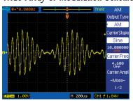
The built-in arbitrary waveform generator is capable of many different types of modulation for various applications. Modulate your waveforms with AM, FM, FSK, PSK, and PWM modulation schemes and use any of the 30 built-in waveforms as the modulating waveform.
