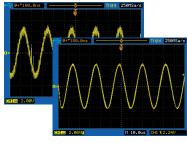
Filter out unwanted signal components such as various types of noise with built-in digital filters. Choose from Low-Pass, High-Pass, Band-Pass, and Band-Stop filters.
