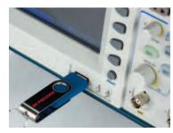
Save and load arbitrary waveform data in CSV format from a USB flash drive.
