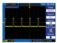
Monitor and analyze long-term signal behavior by recording data continuously over an extensive period of time and playing it back for post acquisition analysis. Data is recorded in a sequence of up to 1000 frames.
