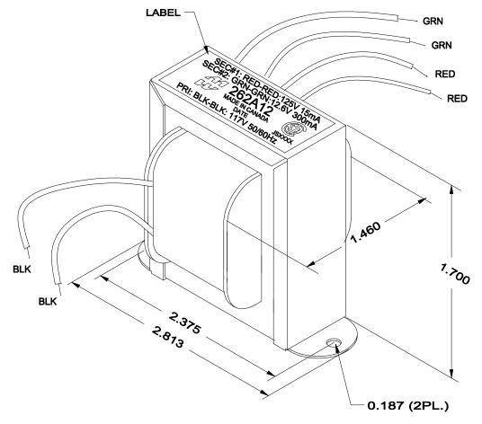
NOTE: ALL LEADS 6" OUT MIN. DIMENSIONS TOLERANCE: ±0.063"
