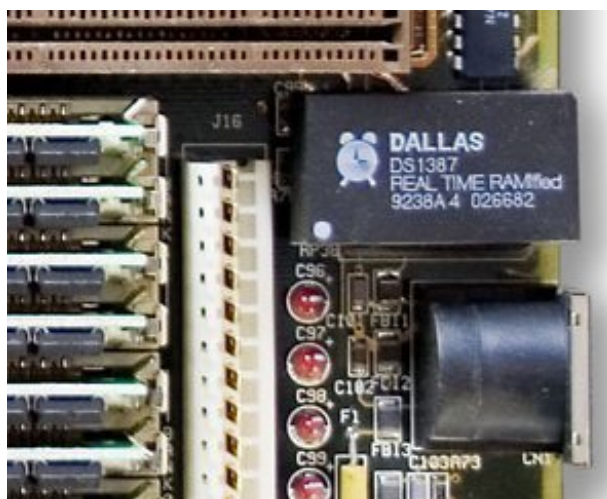
The image above shows a computer motherboard with a Real Time Clock called the
