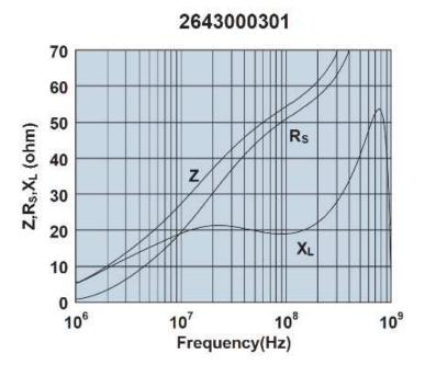
Impedance, reactance, and resistance vs. frequency.
