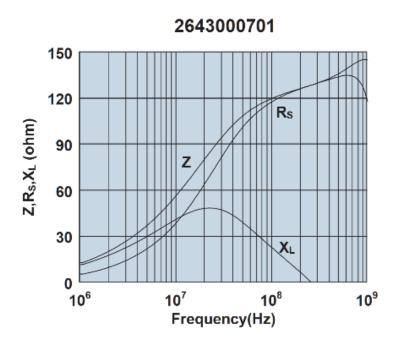
Impedance, reactance, and resistance vs. frequency.
