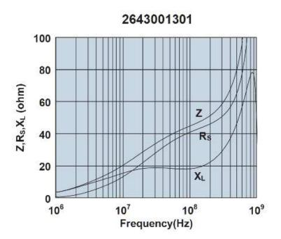
Impedance, reactance, and resistance vs. frequency.
