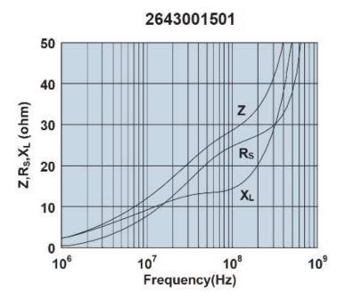
Impedance, reactance, and resistance vs. frequency.
