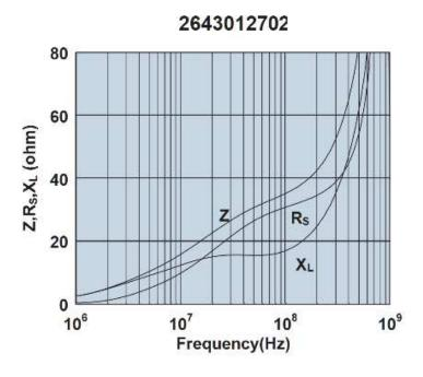
Impedance, reactance, and resistance vs. frequency.
