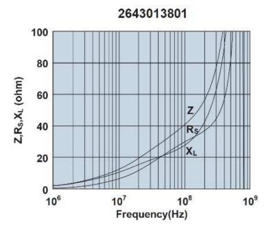
Impedance, reactance, and resistance vs. frequency.
