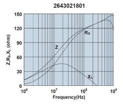
Impedance, reactance, and resistance vs. frequency.
