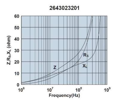
Impedance, reactance, and resistance vs. frequency.
