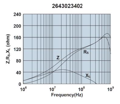
Impedance, reactance, and resistance vs. frequency.
