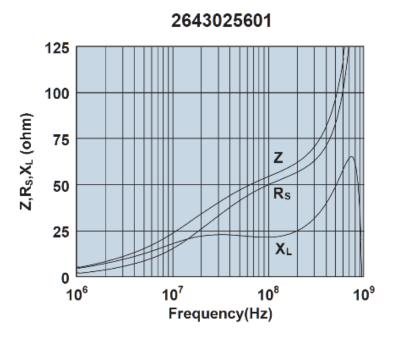
Impedance, reactance, and resistance vs. frequency.
