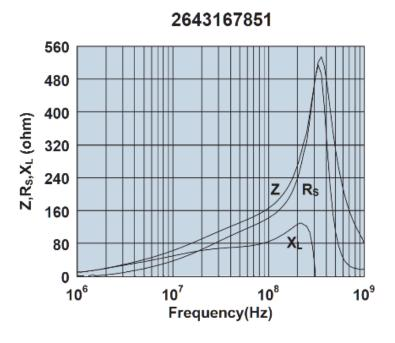
Impedance, reactance, and resistance vs. frequency.
