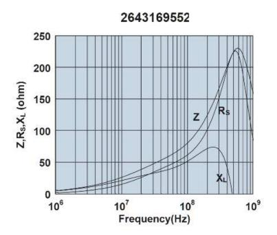
Impedance, reactance, and resistance vs. frequency.
