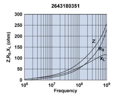
Impedance, reactance, and resistance vs. frequency.
