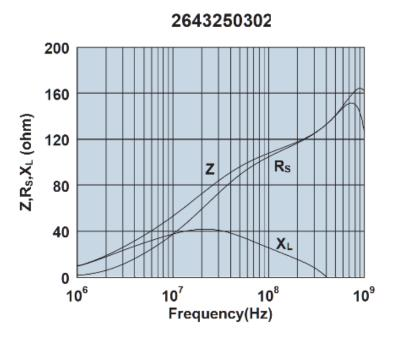
Impedance, reactance, and resistance vs. frequency.
