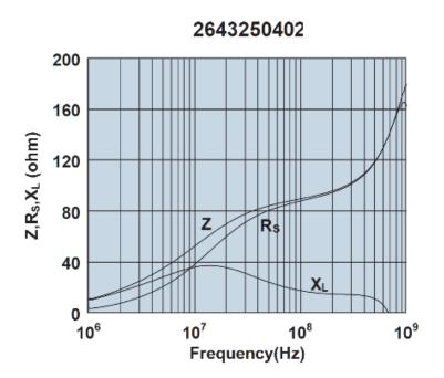
Impedance, reactance, and resistance vs. frequency.
