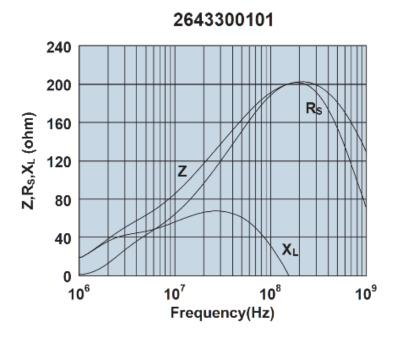
Impedance, reactance, and resistance vs. frequency.
