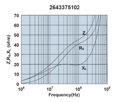
Impedance, reactance, and resistance vs. frequency.
