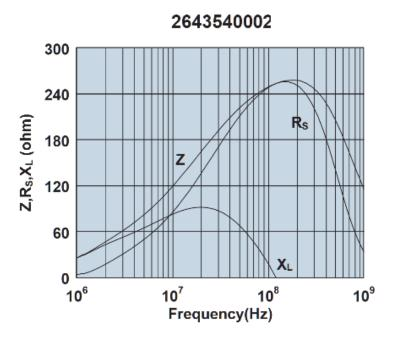
Impedance, reactance, and resistance vs. frequency.
