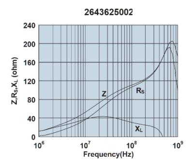
Impedance, reactance, and resistance vs. frequency.
