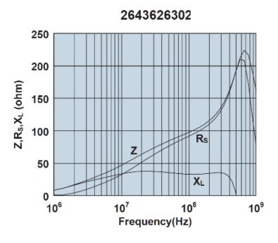
Impedance, reactance, and resistance vs. frequency.
