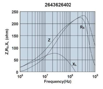
Impedance, reactance, and resistance vs. frequency.
